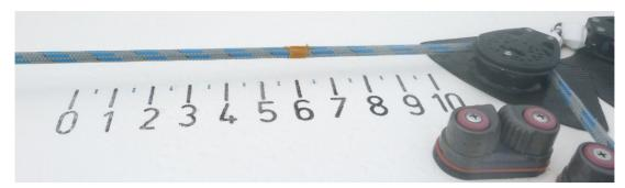
• **Jib Sheet Reference Marks.** We recommend marking the jib sheets with reference marks The first pair of marks will be a close reference and seen in front of the turning block on the leeward side for repeating fast settings. You can combine this with trimming to the spreader reference mark on each tack upwind. Make sure the clew block strop is positioned evenly so the blocks are the same distance from the jib clew when under load.
