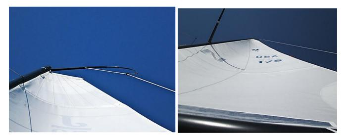
• **Backstay Setup.** After shrouds are tensioned for the conditions, make sure the backstay bridle is just slack when it's not cleated. As the wind speed increases, the backstay bridle should be shortened to take most of the excess slack out of the backstay before tensioning so you will not bottom out the backstay too quickly as the wind speed increases. Conversely when the wind is lightening, make sure to ease the backstay bridle so headstay does not get too bound up in the light spots.
