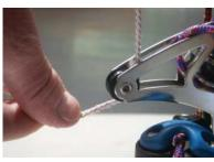
Thread the V12, previously attached 5 to the top block, through the pulley/becket from the top.
