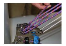
Continue to feed the Dyneema control line back up to the double block, feeding the line from front to back.
