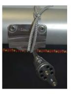
1 Put the top block and tang onto the boom and tie the small length of shockcord in a loop as shown to stop the top block from coming off the boom unintentionally.
