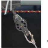
2 Tie the length of Vectran V12 (1.45 m) in a bowline loop through the top block.
