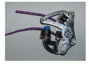
3 Take the length of Dyneema race control line (4.5 m) and thread it through the Harken base unit before you attach it to the mast as shown. Ensure that the tail is underneath the horizontal pair of blocks.
